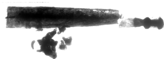
Fig. 20 Radiograph obtained at 80 kV, 2.5 mA, 10 s.
